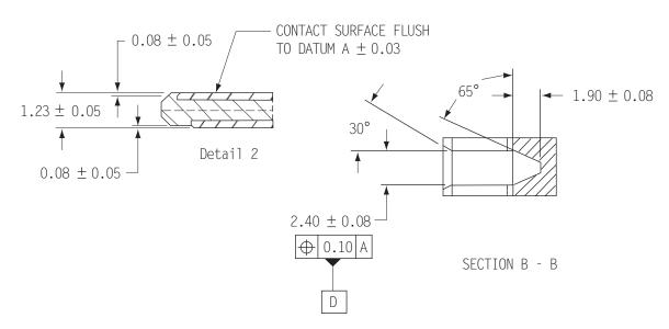
Figure 15. SAS device plug dimensions (detail)
